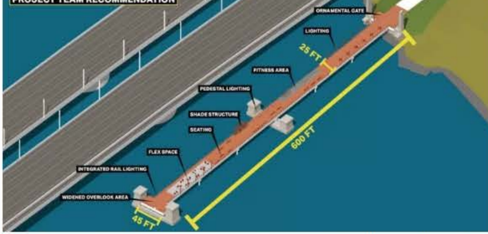
Several piers remaining from the old eastern span of the original Bay Bridge will be reused as a vista point and boardwalk at Yerba Buena Island and Oakland. (Courtesy Caltrans)
