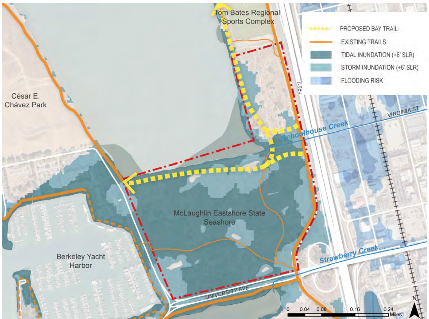
FIGURE 4-18: McLAUGHLIN EASTSHORE STATE PARK End-of-Century - 6ft SLR
